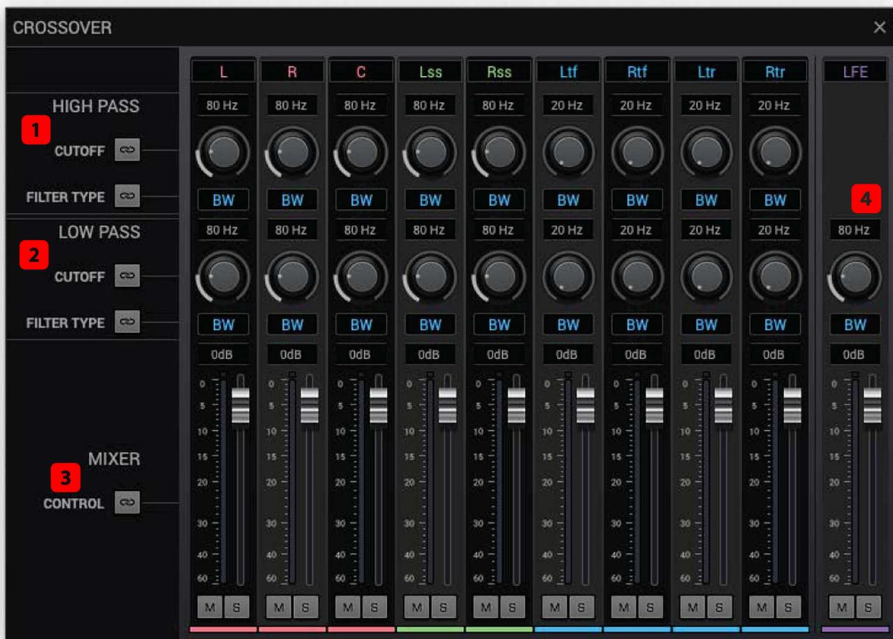
The above mixer is available via the LFE channel settings (LFE crossover button). It provides all bass management settings allowing monitoring low frequency content of the surround/overhead channels via the LFE channel. Global on/off for the crossover is available, again via the LFE channel settings.
