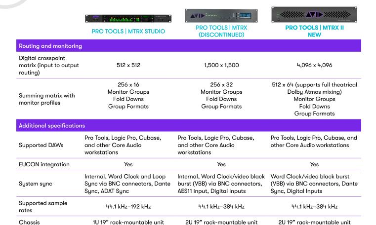
Please note: All digital audio format channel counts are listed at 44.1/48 kHz and are subject to standard channel count reductions at higher sample rates unless otherwise noted.
